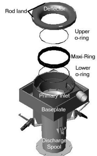
Maxi-Ring 'O' ring (09) around the Maxi-ring locator stub groove provided in the primary inlet (05).
